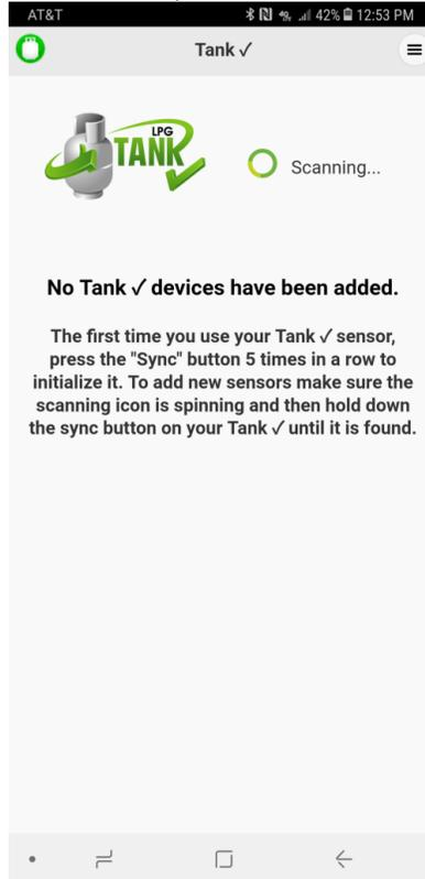
3. Press and hold SYNC button until sensor appears on app. (up to 10 seconds)
